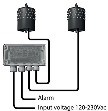
1-4 Navilite 48V working simultaneously
